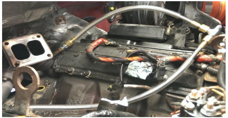
Stainless lines installed with tee fitting
